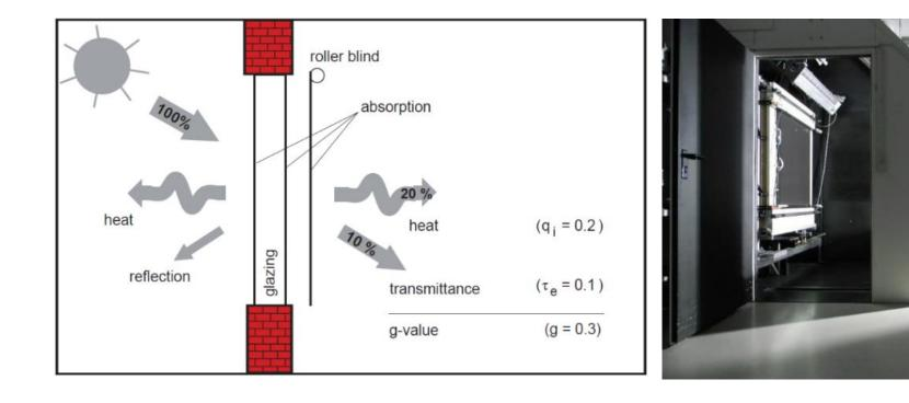
Solar calorimeter for g-value determination of facade components at Fraunhofer ISE
